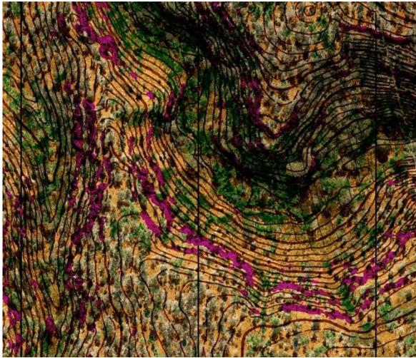
The area was specially flown for LIDAR together with aerial photography at a very large scale. The base map was generated using the default settings distributed with the Pullautin software. These settings are what Jarkko Ryyppo considers to be the most applicable to Finnish terrain. These same settings were used for Transit Flat and except for the identification of boulders were generally acceptable.
