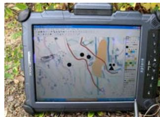
Drawing on iXplore tablet PC with photogrammetry as template
