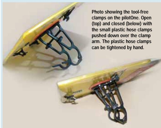
Photo showing the tool-free clamps on the pilotOne. Open (top) and closed (below) with the small plastic hose clamps pushed down over the clamp arm. The plastic hose clamps can be tightened by hand.
